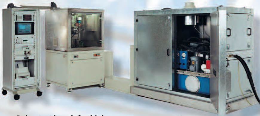
Pulse test bench for high-pressure components
