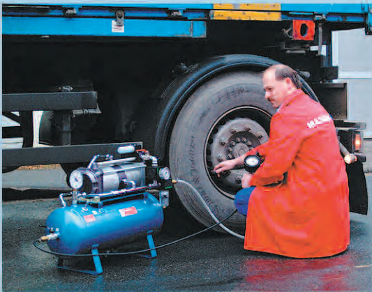
Filling of tyres with 16-bar pressure.
